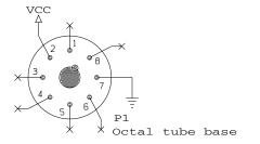
Replacement for Amperite type #6-4 ballast tube as used as R-32 in AF Amplifier AM-65/GRC (Fed Tele & Rad part/dwg #GH-2677-2)
